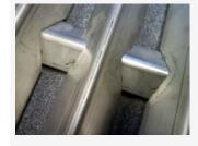
Brand new Flavorizer Bars will be shiny and clean, like the ones pictured above, but it won't take many uses of the grill for them to take on a less attractive appearance. Shown below are the same Flavorizer Bars from the last picture, about a year later. They've developed a bit of surface corrosion, but all they need is some maintenance, and are actually in good condition to keep serving their function.
