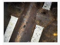
Many people often think that they need to replace their Flavorizer Bars when they develop some surface corrosion, but so long as they haven't developed any holes or cracks in them they should work just fine. The Flavorizer Bars in the next photo are examples of ones that should be replaced.
